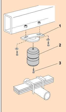
Do not exceed vehicle manufacturer's recommended axle weight rating. Check for AEON® interference with vehicle components - Under load AEON® will "expand" in diameter.
