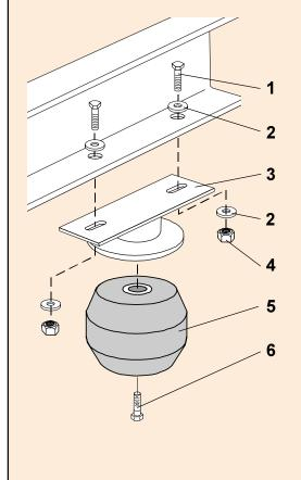
Do not exceed vehicle manufacturer's recommended axle weight rating. Check for AEON® interference with vehicle components - Under load AEON® will "expand" in diameter.
