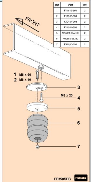
Do not exceed vehicle manufacturer's recommended axle weight rating. Check for AEON® interference with vehicle components - Under load AEON® will "expand" in diameter.
