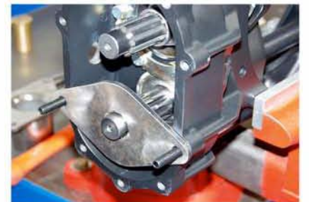
This little tool holds the jackshaft while you tighten and torque the yoke nut.
