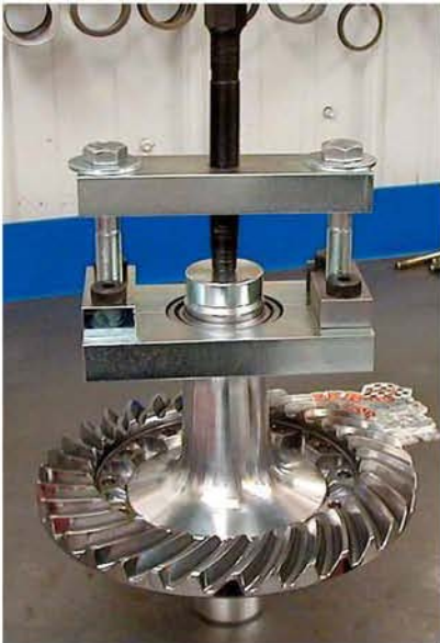
Once the rearend has been bolted together and re-checked for gear lash, a final adjustment might be needed. That means the carrier bearings must be pulled. This tool pulls the pressed-on bearings without causing damage.
