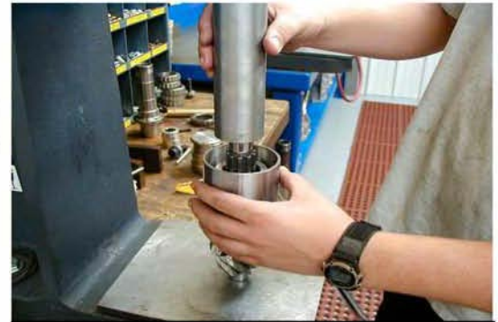
Special tools are used to press the bearings onto the pinion shaft. These ensure that the bearing goes on straight and is properly seated.
