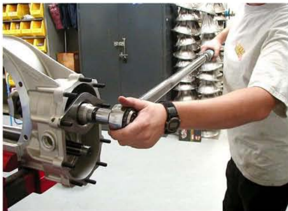
The pinion nut is held in place using a special tool that is held by the cover studs. Then, the pinion shaft is rotated to obtain the proper torque on the nut.
