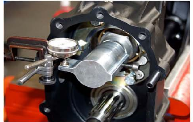
Another unique tool is this pinion flag tool. It is specially designed to provide a surface on which to rest the dial indicator while checking for gear backlash. The distance from the center of the pinion shaft to the point where the indicator lies is the same as the distance to where the gears mesh. This way you get a true lash measurement, just as if you had measured between the actual gear teeth.
