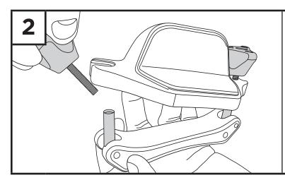
• Attach two 3-wing knobs with bolt to Flip-Fit bracket.
