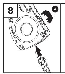
Feed end of rope up through the bottom while rotating the spool clockwise.
