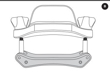
• The Flip-Fit bracket can be rotated and flipped to fit different width load bars. The tips on the Flip-Fit bracket should face down to fit thinner load bars (Figure A) and up to fit wider load bars (Figure B).
