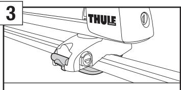
• Wrap Speed-Link rubber strap under load bar and place T-end into pocket on end. Repeat with other 3 Speed-Link straps.
