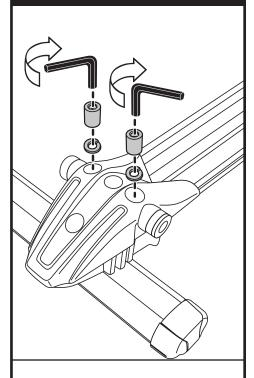
Assemble lock washers and nut to square head bolt as shown. Drop washers and round nuts in holes first. Tighten with hex key.
