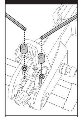
• Assemble lock washer, and nut (included with Echelon) to square head bolts.
