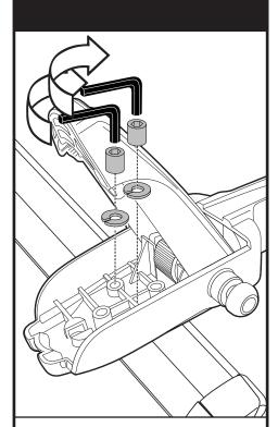
Assemble lock washers and nut (included in Peloton hardware) to square head bolt using center holes.
