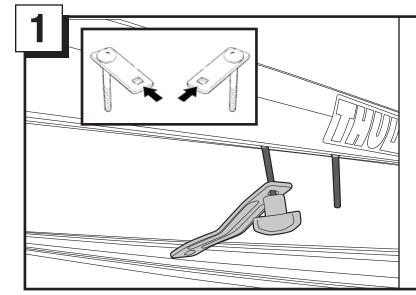
Using the two rectangular plates that are included with the fork mounted carrier-install one bolt in the ends, slide the plates into the slot in the bottom of the wheel tray, leaving the empty holes in the middle.
