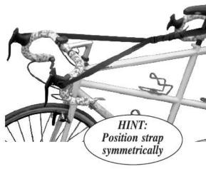
Remove and stow front wheel (Recumbents: also remove seats)
