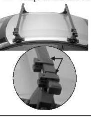
B Loosen nuts to adjust rear bracket
