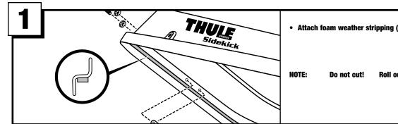
• Attach foam weather stripping (F) to inside flange of Carrier top.
