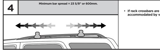
• If rack crossbars are adjustable, set to widest position which can be accommodated by vehicle and box's mounting points.
