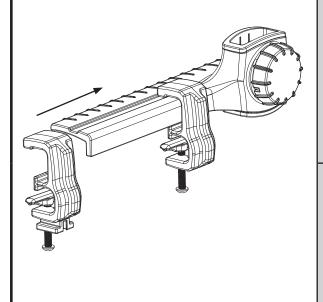
NOTE: If having trouble getting top of Clamp to slide onto Base Assembly, apply pressure to Base Assembly so that it compresses down onto bed rail.
