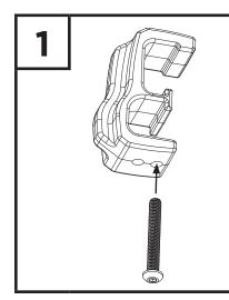
• Thread BHCS into bottom, front hole of Clamp and place Clamp Foot on top of BHCS.
