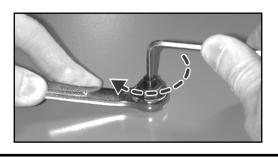
• Remove flaring tool by holding nut with %" wrench and turning screw counter clockwise.
