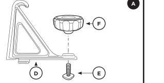
1. Pre-assemble all load stops as shown. Attach knob loosely.
