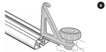
2. Slide tiedown into top crossbar track (A), locate in desired position, and twist knob until securely in place.
