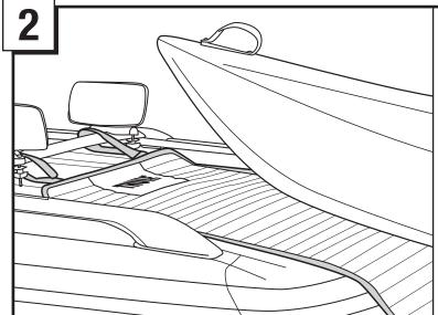
The kayak/canoe may rest on the Waterslide mat and be slid across the mat during loading and unloading. The mat's fabric surface will help the boat glide into the carrier and prevent damage to the vehicle.
