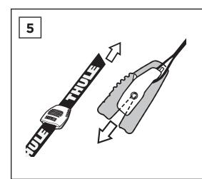
Route free end of strap, with logo side up, through the Buckle Bumper as shown. Pull Buckle Bumper over buckle to protect boat and vehicle while strapping down boat.
