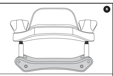
• The Flip-Fit bracket can be rotated and flipped to fit different width load bars. The tips on the Flip-Fit bracket should face down to fit thinner load bars (Figure A) and up to fit wider load bars (Figure B).
