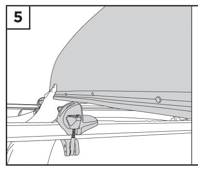
Lift canoe, turn upside down and place canoe gunwales onto cushioned grey pads of base. Loosen knobs and adjust spacing of bases on load bar to fit canoe properly. Tighten all eight knobs firmly so that bases do not move.
