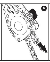
Keep rotating the spool until rope exits at the bottom.
