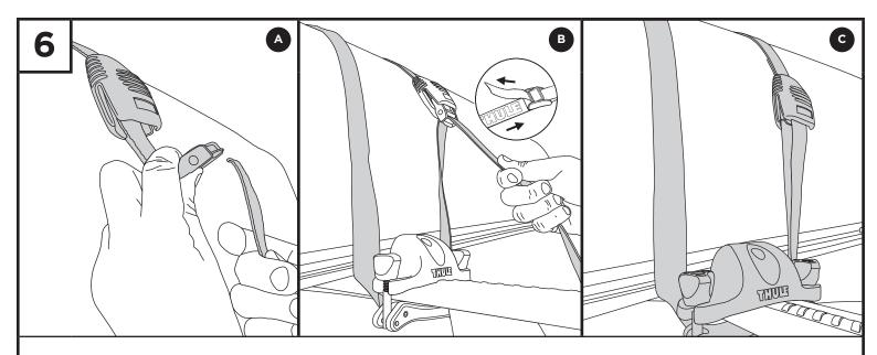
Wrap strap over canoe and under load bar on both sides of canoe. Slide buckle bumper over metal buckle to prevent vehicle and canoe scratches. Thread end of strap through metal buckle by pushing down on lever and then pulling down to tighten. Re-cover buckle with buckle bumper.
