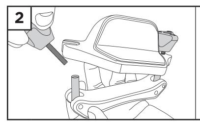
• Attach two 3-wing knobs with bolt to Flip-Fit bracket.
