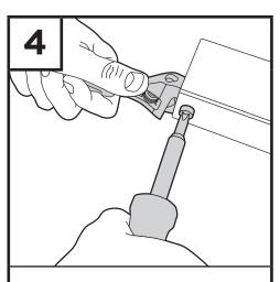
With Phillips head screw driver and adjustable wrench, remove safety bolt.
