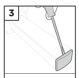
Remove end cap from opposite end of tubing where rear wheel holder is located.
