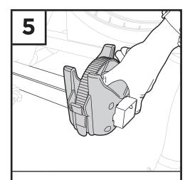
Slide Fat Tire rear wheel holder onto tube. Make sure buckle is facing out, away from vehicle. Reattach safety bolt and end cap.
