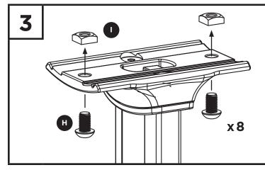
Insert 5/8" Button Head Cap Screws (H) through bottoms of Saddles and thread <u>loosely</u> into Square Nuts (I). Make sure flat sides of Square Nuts are facing down towards Saddles.
