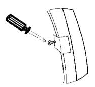
C. Once serew is in position inside wheel well and making sufficient contact with inside of vehicle fender, tighten the screw carefully against the fender underside. Screws should be tightened just enough to secure trim Firmly in place.
