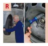
To prevent wheel hub damage and / or lateral run-out of the brake discs, the wheel bolt / nut must be tightened according to the manufacturer's specifications (sequence + torque).
