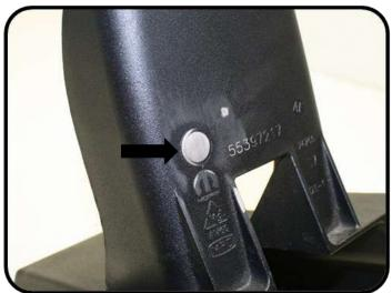
Use the factory screws to position the extension bracket as pictured. Use the holes closest to the middle of the extension bracket.
