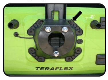
4. With the mount removed, grind off the small bump on the back of the mount.
