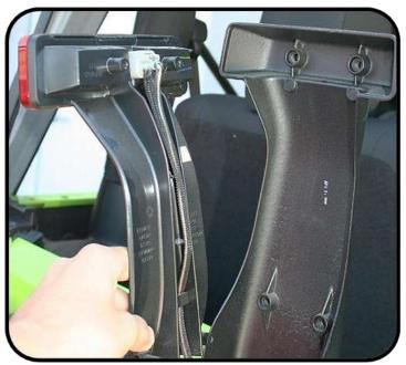
3. Remove the factory tire mount from the vehicle by unthreading the eight bolts that secure it.
