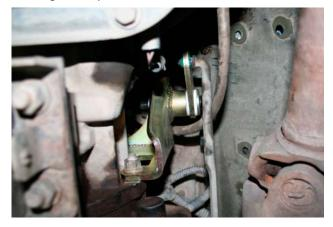
5. Remove the plastic bushing from the shift lever that sticks down through the floor of the body tub. (photo)
