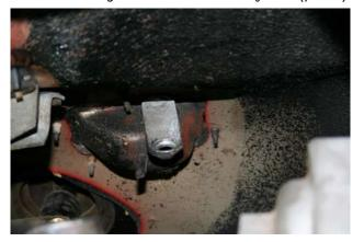
**Note:** We recommend using loctite® on the shift linkage nuts.
