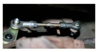
**Note:** We recommend using the "neutral" position of the transfer case as the starting point. Put the shift lever in the neutral position as well as the transfer case. Adjust the linkage accordingly.
