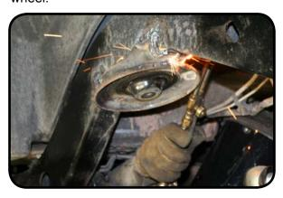
25. Grind the frame flush so that the new TeraFlex Speedbump coil perch mounts correctly.
