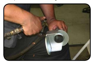
29. Tack the bracket into place. Make sure that the bracket lines up to the axle. Once you have the bracket located correctly weld it in completely and paint all of the welded or raw areas.
