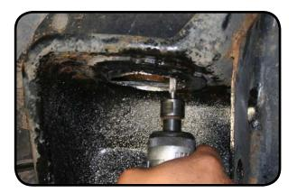
11. After you have cut though both layers grind the jounce tube flat to ensure a good fit and weld with the new Speedbump bracket.
