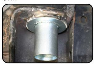
Once the bracket is in its final location, finish welding it into place. Paint all of the welding areas.
