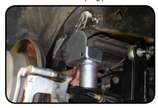
27. Mark around the mount. This will be where you need to prep the frame for welding.
