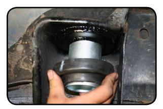
16. Smear silicon onto the Speedbump to protect it from water entering the void in between the Speedbump and the mount.
