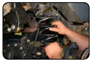
4. Remove the bump stop by pulling it away from the frame.
