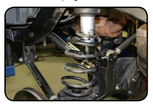
35. Reinstall the shocks, sway bar links and track bar if they were removed.
