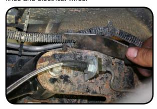
24. Cut off the old coil perch using a torch or cut off wheel.
