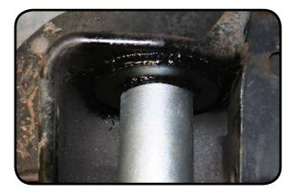
15. Install the new coil spring isolator.
