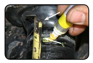
8. Cut the jounce tube with a cut off wheel, this cut is made to locate the hole saw. You may need to pry the jounce tube towards the frame to completely cut through the tube.
