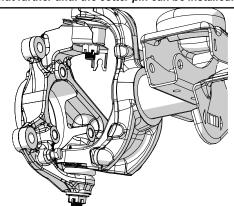
Now is a great time to grease the upper and lower ball joints with a premium grease before reinstalling the remaining components. Fill the ball joints until you can feel the boots begin to slightly swell. **DO NOT OVER-FILL**.
