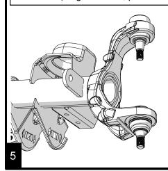
Remove the upper, then the lower ball joints, using a ball joint press.
