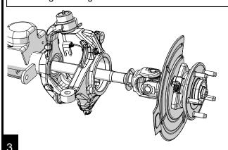
Remove the cotter pins and loosen the upper and lower ball joint nuts but do not completely remove. This will prevent the knuckle from falling off when it breaks loose from the ball joints.
