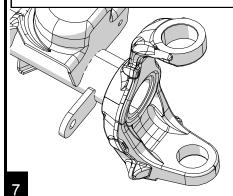
The orientation for the passenger side of the Jeep is opposite of the driver side. Note: The set screws must face the tire for access.
