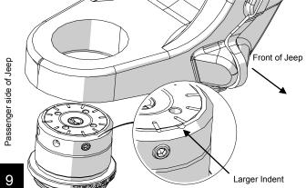
Install the new TeraFlex upper ball joints.
