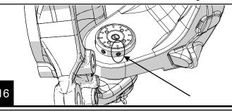
Insert supplied grease zerk extension in the set screw hole and lightly tighten. Insert supplied grease zerk into the extension and tighten. Grease as needed. Remove the Grease Zerk Extension assembly and replace the set screw with blue Loctite before vehicle use!
