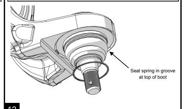
Install remaining set screws to seal the ball joint. Put a drop of blue Loctite on the threads before installation.
