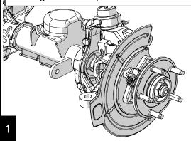
Remove the three 12 point 13mm bolts that secure the unit bearing to the outer knuckle. Repeat on opposite side. Be sure to unbolt and remove the ABS sensors from the outer knuckles before moving onto step 3.
