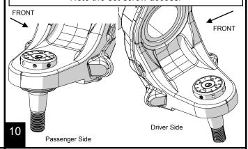
Reinstall the lower ball joint boots and install the boot retaining springs.
