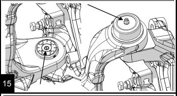
Alternate method of greasing the TeraFlex Lower Ball Joint: Locate and remove the set screw that has a positioning slot aligned with the cap. This must be either the most forward, or most rearward set screw for the grease zerk extension to clear the outer knuckle, when the knuckle is turned left or right, depending if the most forward or rearward set screw is aligned.
