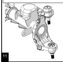
Remove the boots from the new TeraFlex lower ball joints to prevent damage. Orient the ball joint as shown for the drivers side.
