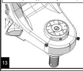
Reinstall the outer knuckle to the ball joint studs. Don't forget the ABS wiring retainer. Torque the upper and lower ball joint nuts to 70 ft-lbs (95 N-m).
