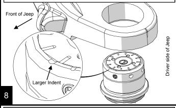
Press the lower ball joint into the inner C.
