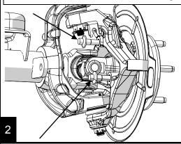
Remove the unit bearing and axle assembly. Support the inner axle shaft so that the inner axle seal is not damaged during removal. Remove dust shields.
