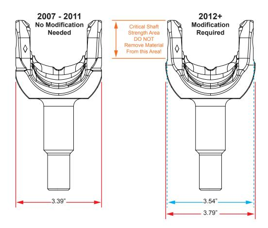
2012 and newer front Dana 30 & Dana 44 equipped JK Wranglers utilize a larger diameter outer stub shaft. This causes interference issues when used with TeraFlex HD Ball Joints (lower ball joint only).
