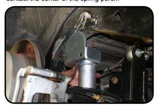
27. Mark around the mount. This will be where you need to prep the frame for welding.
