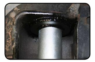
15. Install the new coil spring isolator.
