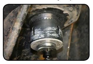
10. You may need to use a die grinder to open up the hole to get the hole saw to cut through the second layer.
