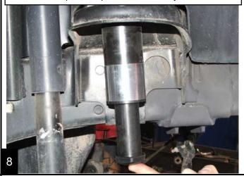
Remove the speedbump and center the strike pad on the spring perch. Use a center punch though the hole to mark the center.
