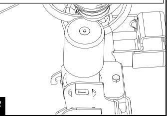
Install the washers and nuts. Torque to 30 ft-lbs. For 3"-4" kits, install is complete.
