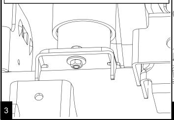
For 6" Applications Only: Remove the factory bumpstop from the cup on the frame by twisting and pulling to the side.
