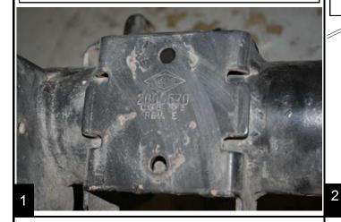
Install the speedbump with the cylinder towards the front of the vehicle. The studs will install into the factory holes in the axle bracket.
