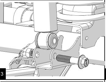
Remove the lower shock nut and bolt with an Tomm.
