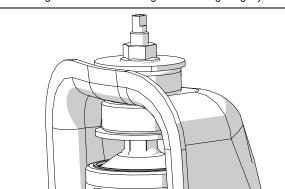
Reinstall the bolt and nut, torque to 56 ft-lbs.
