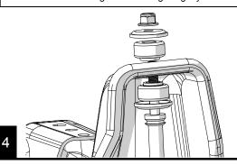
Reinstall the two lower bolts and nuts, torque to 21 ft-lbs.
