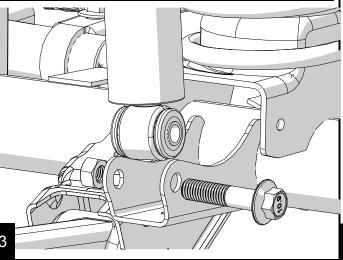
Remove the lower shock nut and bolt with an Tomm.
