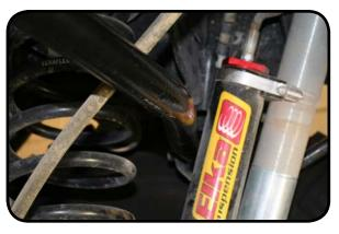
4. Adjust the track bar so the axle is centered under the vehicle. Torque the collar pinch bolts to 80 ft-lbs using an 18mm socket and wrench.
