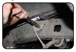
10. Carefully lower the rear axle far enough to remove the rear springs. Be careful not to let the coils fall out as you lower the axle. You will want to lower the axle far enough to install the new 1.5" springs in place. While lowering the axle make sure the brake lines, ABS wires and axle vent do not stretch as this could cause damage to these vital parts.
