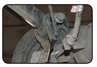
8. Remove the bracket that holds the park brake cables to the body using a 10mm deep well socket.
