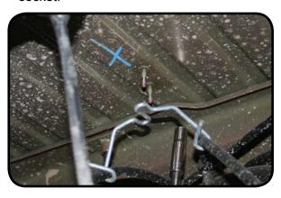
9. Remove the brake line mount at the frame using a 10mm socket.
