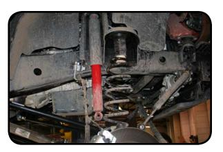
18. Remove sway bar links using 18mm socket and wrench at the axle and 18mm socket and 20mm wrench at the sway bar. Lower the jack enough to remove the springs.
