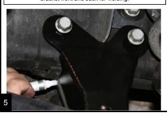
Place the new frame brace bar with the fixed end side into the factory trackbar location with the bend of the bar upwards. Insert a 9/16"x3.5" bolt into the top hole.
