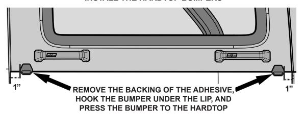
THESE BUMPERS ALLOW YOU TO PLACE THE HARDTOP ON THE GROUND WITHOUT THE RISK OF DAMAGE. PLACE THE BUMPERS ABOUT 1 INCH FROM THE OUTER EDGES.
