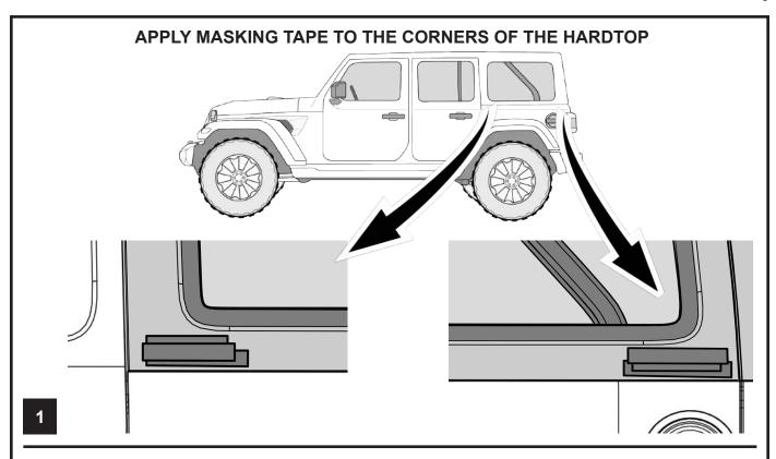
TAPE THE TEMPLATES TO THE CORRESPONDING CORNERS OF THE HARDTOP
