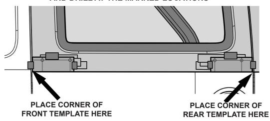
USE A TAPE MEASURE TO VERIFY THE POSITION OF THE HOLE MARKERS.
