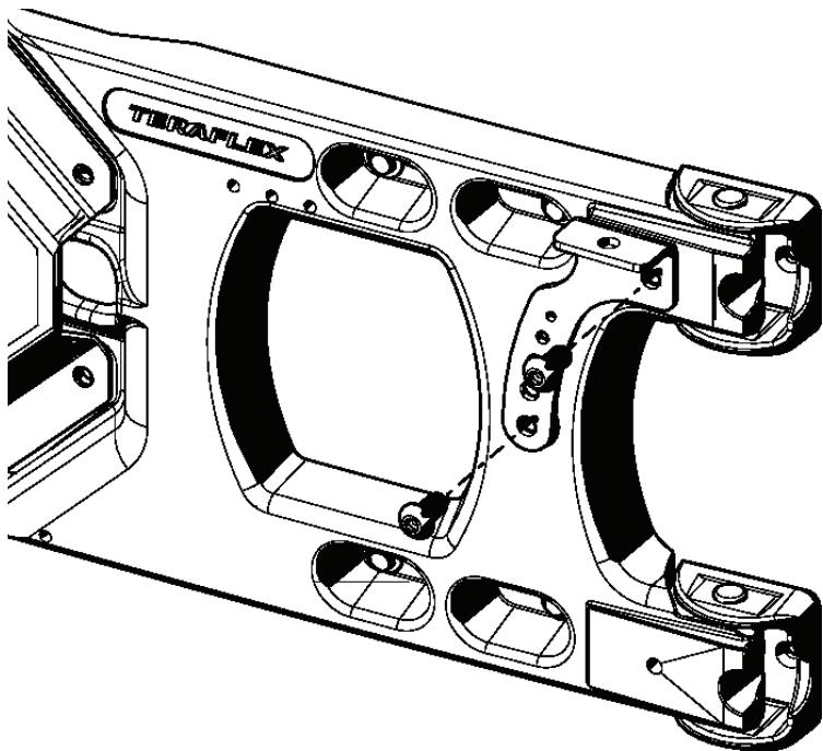
2. Insert the two  $\frac{1}{2}$ "-13 bolts through the CB Antenna Mount and thread them into the aluminum tire carrier. Torque to 55ft. Lbs.
