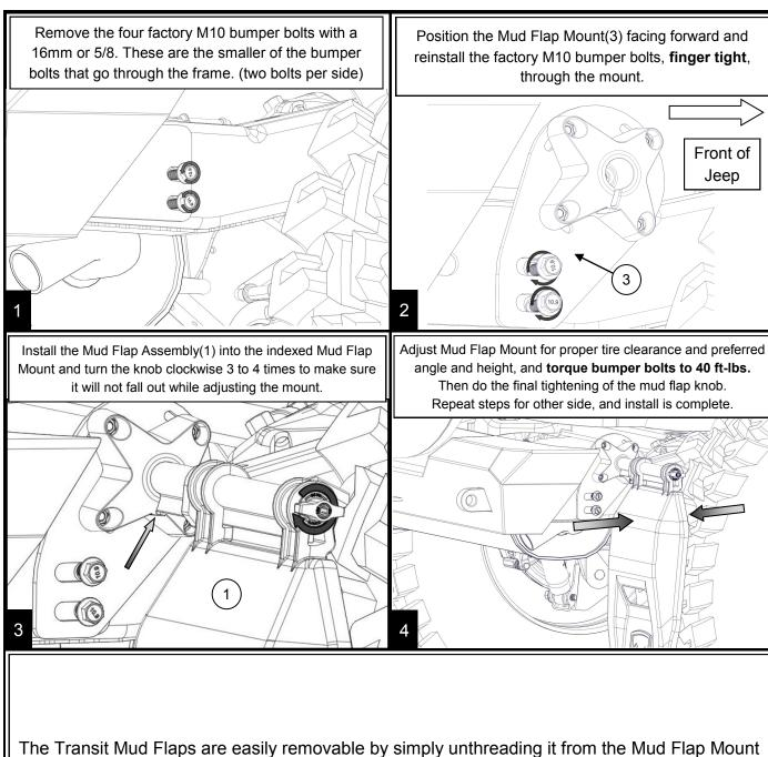
The Transit Mud Flaps are easily removable by simply unthreading it from the Mud Flap Mount using the Mud Flap's end Knob
