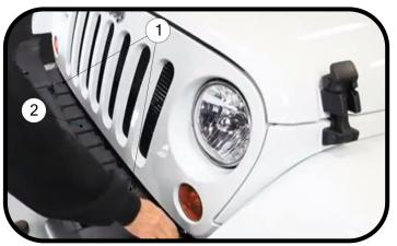
Remove the font splash shield (3) by removing the 4 push pin fasteners(1) connecting it to the bumper the 2 push pin fasteners (4) that connect it to the frame behind the splash shield.
