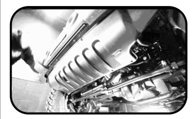
10. Using the phillips screwdriver, remove the 4 screws(3) on each fog light and remove the fog lights from the rear bumper.
