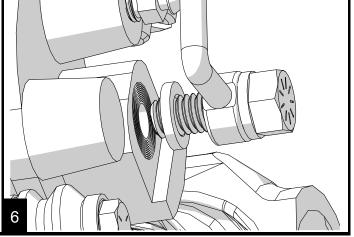
Orient the brake line as shown and torque the banjo bolt to 23 ft-lbs.
