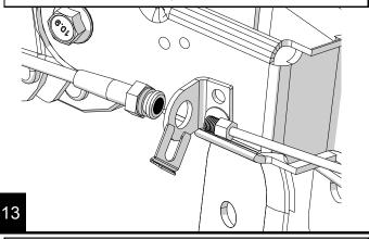
Hand tighten the hard line into the new line.
