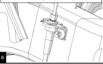
Use a 10mm end wrench and break loose the brake line before removing the frame bracket with a T40 torx.
