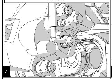
Make sure the line will not snag on any components when the suspension moves and when the tire turns. Then torque the hard line to 12 ft-lbs. If you are only installing the front, bleed the brakes using standard bleeding procedures.
