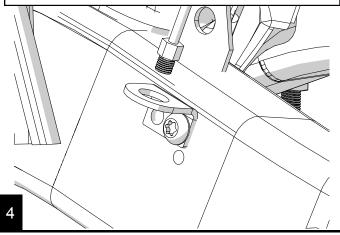
Install one of the copper washers on each side of the banjo fitting and reuse the origional banjo bolt.
