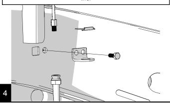
Orient the line as shown on the caliper. Torque banjo bolt to 23 ft-lbs.
