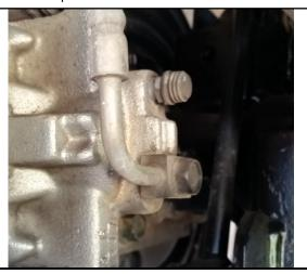
Remove the brake line from the hard line with a 12mm.
