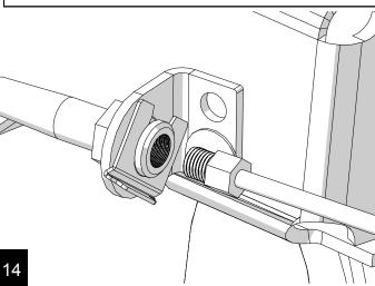
Install the T end of the line to the axle with the breather tube. Reinstall the hard lines into the T. Torque to 12 ft-lbs.
