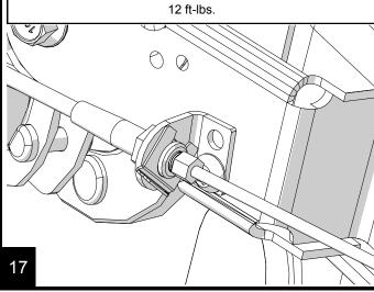
Bleed the brakes using standard bleeding procedures.
