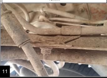
Disconnect the two hard lines at the T on the axle housing. The breather is used as the brake line retainer. Remove with a 9/16".
