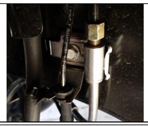
Place a new copper washer on the banjo bolt and insert though the end of the brake line. Place another copper washer between the fitting and the caliper.
