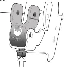
Insert the supplied M12 x 70mm bolt through the middle opening followed by a washer and M12 nut. Hand tighten.
