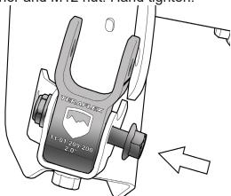
Reuse the factory hardware to mount the shock into the extension. Torque the bolts starting from the bottom to the top.
