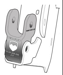
Align the extension in the axle mount and insert the supplied M12 x 20mm bolt. Hand tighten.
