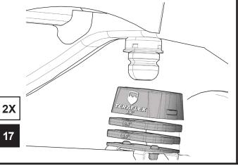
INSTALL THE BUMPSTOP ASSEMBLY ONTO THE MOUNTING PLATE
