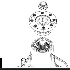
Check the torque required to rotate the pinion and increase the pinion nut torque in 5 ft-lb increments until the torque required to rotate the pinion is back to the original measured value.
