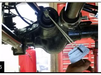
Apply a bead of silicone to the splines of the new yoke. Install the yoke onto the pinion. Apply red thread locking compound to the threads of the provided pinion nut and torque to 160 ft-lbs.
