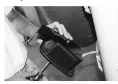
Position the antenna mounting bracket between the vehicle and the tail light housing. The mounting portion of the bracket will be positioned towards the outside edge of the tail light housing when properly installed.
