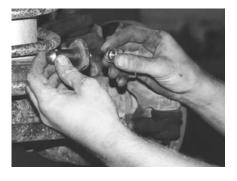
**Step 3**Use the pin for leverage when tightening the nut with a 3/4" wrench.
