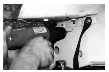
**Step 6**Attach the retention strap hook to the vehicle using the included metal screws.
