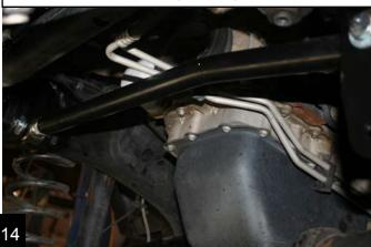
Using a 13/16" drill bit, drill out the knuckle and tap the new taper sleeve in from the top. Be sure to drill straight.
