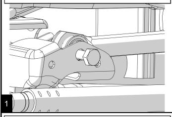
Remove the factory drag link at the knuckle by loosening the 21mm castle nut and hitting the face of the knuckle with a hammer. This will break the taper loose. Then remove the nut.
