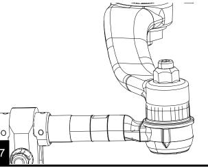
Install the new drag link to the knuckle. Flip drag link end applications require using a lock washer as a spacer between the nut and the knuckle. Full replacement flip drag links do not. Torque to 65 ft-lbs. Re-torque all ball joints after 200 miles.
