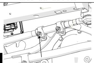
If you purchased the premium drag link as part of this kit, remove the drag link completely. Loosen the nut at the pitman arm and strike the face with a metal hammer to release the taper. Remove the nuts and the drag link.
