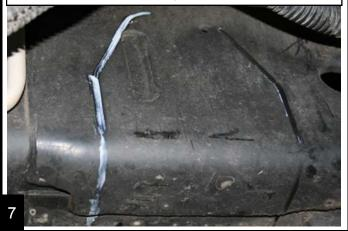
When the desired location is established, remove and prep the brackets and frame for welding. Clean the frame and brackets with a sand pad or wire wheel. Clean surfaces are crucial to a good structural weld.
