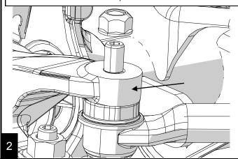
If you purchased the premium drag link, see step 4. Loosen the drag link side of the adjuster sleeve with a 15mm.
