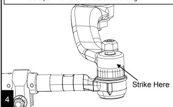
With an 18mm remove the two lower steering box bolts. Install the new drop bracket and tighten the bolts. Mark the bracket front and back for welding.
