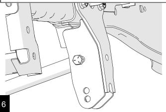
Loosely install the frame side bracket bar using a 9/16 bolt. Position the brace bracket against the frame and mark for welding prep.
