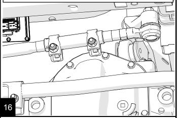
Install the drag link end closest to the adjustment sleeve into the pitman arm. Torque lock nut to 77 ft-lbs (105 Nm)
