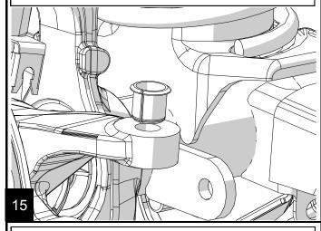
Install the new heavy flip drag link into the adjusting sleeve.
