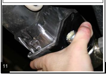
With the brace bar removed, final weld the frame bracket as well as the drop bracket at the steering box.
