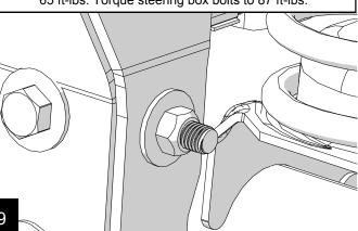
Cut off exposed bolt past the nut with a cut off wheel.
