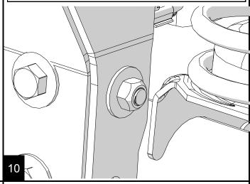
The brackets should be flush against the frame and the cross bar should not be at a bind.
