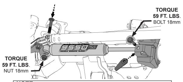
NOTE: CYCLE THE SUSPENSION AND STEERING TO CHECK FOR PROPER SHOCK BODY CLEARANCE AND TRAVEL
