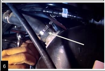
Use a screwdriver or equivalent to depress the white release to disconnect the vent line.
