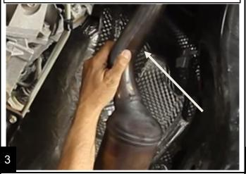
Clean frame and front bracket of paint everywhere you will be welding. Clamp the bracket into place to close any gaps between the bracket and frame. Weld it on.
