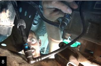
Be sure to cap/protect any open fuel lines. On most models the supply and return lines can be snapped together.
