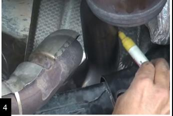
Cut about 2.5" of pipe off of the rear of the converter. Cut as square as possible, you will be reusing this section of pipe.
