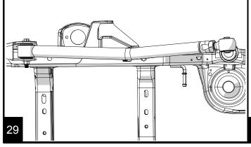
Raise the axle and reinstall the front shocks. (See 999207 Shocks/Front Installation)
