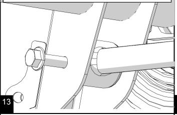
Support the front axle, un-bolt the bottom of the shocks with an 18mm (See 999207 Shocks/Front Removal).
