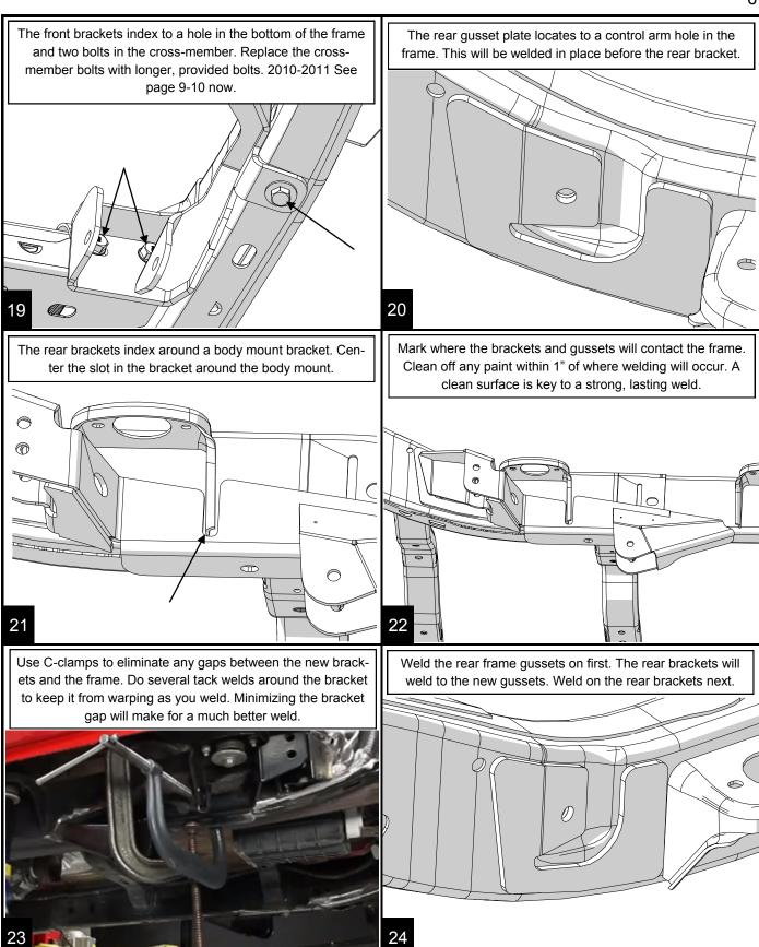
Weld the front brackets. Take some time after welding to clean these sections and paint to prevent rust.
