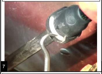
Disconnect the supply and return lines by squeezing the blue tabs. *Caution!* The supply line may still be under pressure. Have a rag ready to absorb any fuel leaks.
