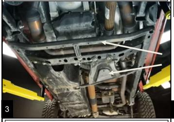
Skip steps 4-5 if you are not replacing the factory drivelines. Make a mark across the flanges at the axles and transfer case. Remove the 8 bolts at each CV end with a 5/16" socket. The front axle end is 4 bolts and a 15mm.
