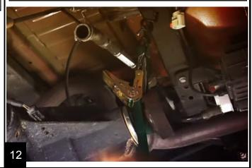
With the axle supported, remove all four rear control arms with a 21mm or an 18mm. Keep the hardware. Most nuts are captured nuts.
