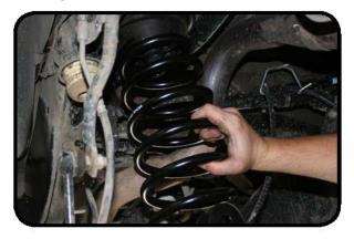
12. Use grease and install new upper spring guide spacer by popping it into the factory location.
