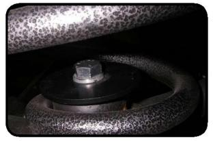
16. Install new rear sway bar links on the inside of the sway bar and the inside of the axle bracket. Use the factory bolt on the axle side with the nut on the outside so excess threads will not interfere with the shock. Use the provided 12mm bolt and washer for the top side with the 12mm nut and washer on the inside to give the most possible room for tire clearance. Torque to 75 ft-lbs.
