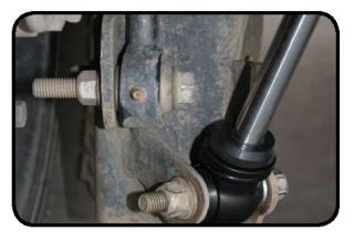
17. Install new rear bump stop spacer by placing the spacer on the axle pad. The extended part of the pad facing forward. Use the provided 5/16" x 1 ¼" bolts with 5/16" washers and 5/16 nuts. Tighten with 1/2" wrenches.
