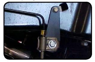
19. Install the new rear track bar bracket by removing the lower control arm bolt. Place the bracket into place, reinstall the control arm bolt. Install the supplied bolt and sleeve into the factory track bar location. Using the supplied u-bolt and nuts install the u-bolt around the axle tube. Torque the u-bolt nuts to 85 ft-lbs and the supplied bolt to 75 ft-lbs.
