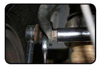
8. Remove the clips that secure the ABS wiring harness to the upper control arm mount.
