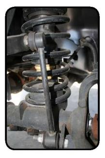
31. Remove the factory brake lines and replace with the supplied brake lines. Use the factory bolt to mount the new tab to the frame. Insert the retaining clip into the brake line as shown.32. Bleed the brakes.
