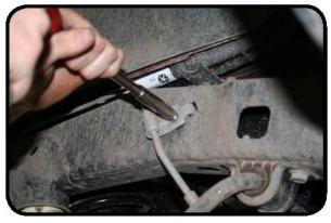
10. Remove the bracket that holds the park brake cables to the body using a 10mm deep well socket.
