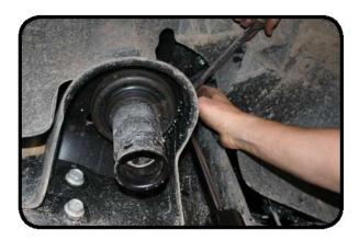
25. Remove sway bar links using 18mm socket and wrench at the axle and 18mm socket and 20mm wrench at the sway bar. Lower the jack enough to remove the springs.
