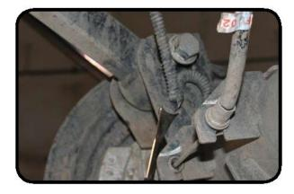
9. Disconnect the brake line bracket at the frame using a 10mm socket. DO NOT DISCONNECT THE BRAKE LINES FROM THE CALIPERS.
