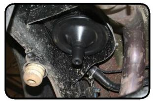
Install the factory isolator on the new spring guide spacer. Don't forget to reuse the factory spring isolator. If the isolator is left out your ride height will be about 1/2 inch lower in the rear. The isolator also helps dampen noise.
