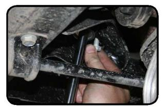
7. Remove sway bar links using an 18mm socket and wrench,
