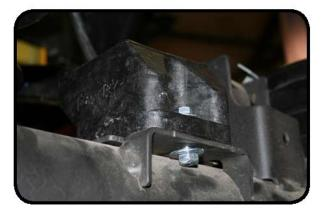
18. Install rear brake line extensions provided in the kit. Bolt the bracket to the factory brake line bracket by removing the 10mm bolt and installing the bracket in that location with the bend of the bracket going flush with the frame. NOT STICKING OUT AWAY FROM THE FRAME. Torque to 14 ft-lbs. (If bracket gets installed the wrong way it will rub on your tires) Then use the supplied hardware to attach the factory bracket to the drop bracket by using 1/2" socket and wrench.
