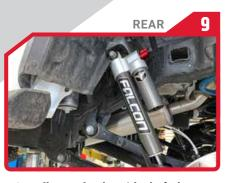
· Install rear shocks with shaft down Shock #1= driver side Shock #2 = passenger side
