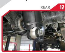
Install the lower end using the factory hardware and torque to 100 ft. lbs.
